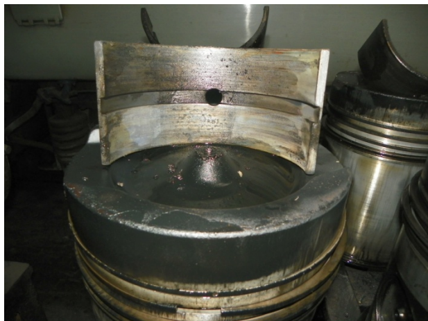
Fig.7 Cuzinet fus maneton arbore cotit
