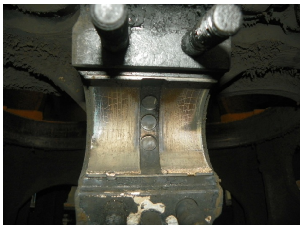
Fig.11 Cuzinet fus ax cu came
