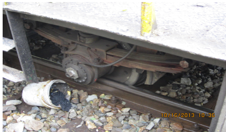
Photo no. 5: The derailed tower wagon DP 58
