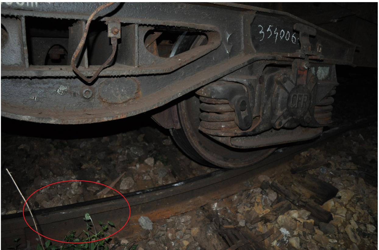
Photo no. 6 - 2 derailment traces on the right side
