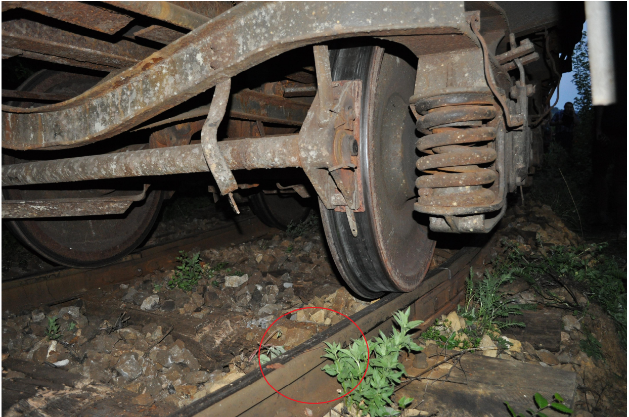
Photo no. 5 - A derailment trace on the right side
