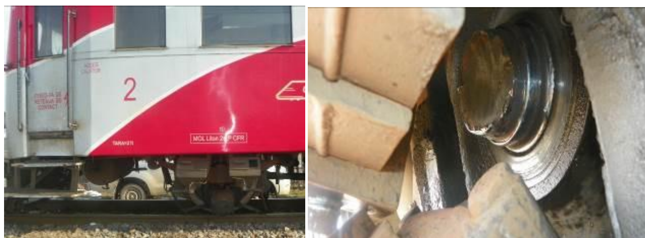
Picture no.1 – breakage of the axle journal on the left side in the running direction, respectively from the short part of the driving axle
